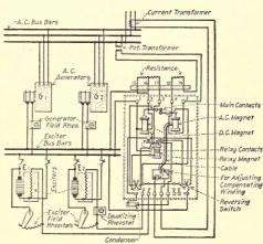
Fig. 194.—Arrangement of an automatic regulator for exciters of small capacities controlling several alternating-current generators in parallel with their exciters in parallel.
